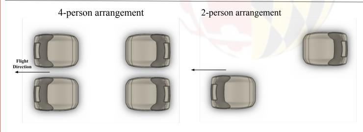
Removable cabin seats allow for safe and easy ingress/egress of passengers with wheelchairs and can accommodate up to 4 fully-mobile passengers without and 2 passengers with reduced mobility
