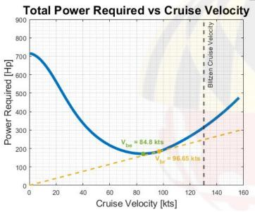
Power Required RotorProp vs Cruise Velocity
